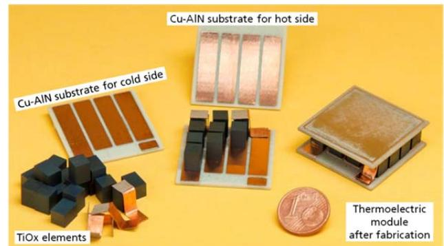
Image 1: Components for TiO<sub>x</sub> based unileg modules
